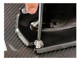
· Continue to hold the mast in place and tighten the bolts with the 5mm hex key.
