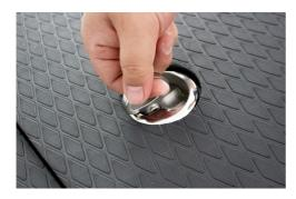
Open the compartment hatch by identifying the hatch compartment compression latches, pressing down on the top of the hatch, lift the latches up and rotate to open.
