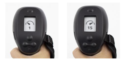
$\cdot$  The home screen of the hand controller displays the battery level of the main battery inside the board, indicating how much ride is remaining.
