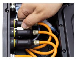
Next, insert the phase connectors by matching the colors and pressing firmly.
