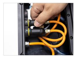
Find the three phase connectors and the blue water tube that were fed into the board when connecting the mast.
