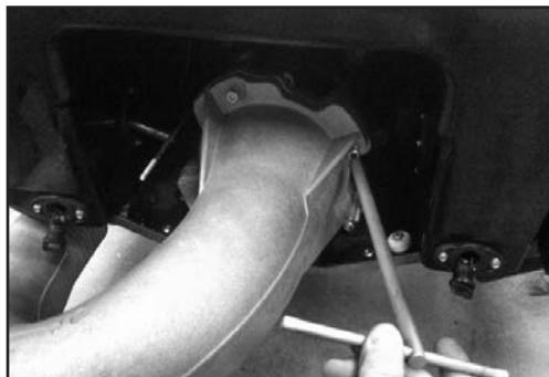
The screws on the outlet elbow (part A01) must be tightened in reverse and moderately (2kg max) because could break the key or screw. Tighten first screw in the top right
